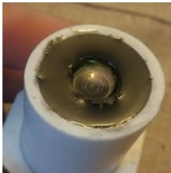
c) Potting material applied.
