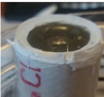
d) Acrylic lens in place with JB weld.
