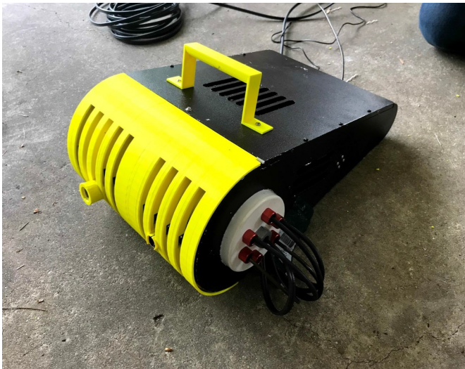
b) PVC cap with cable penetrators and completed ROV.
